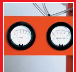
Easy to read pressure and vacuum gauges.
